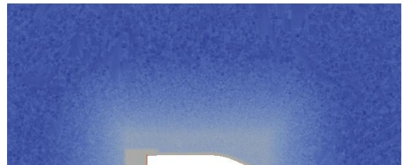
Fig. 5 Indication of the mesh density on the horizontal cut at the free surface level.
